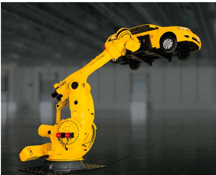
Completed car handling by M-2000iA/1700L
