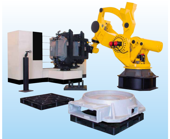
Large casting machine tending by M-2000iA/1200
