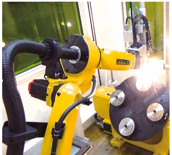
FIBER LASER welding
