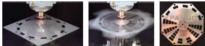
High-speed, high-precision cutting and marking of rotating workpiece ("FANUC" character marking: 120m / min)
