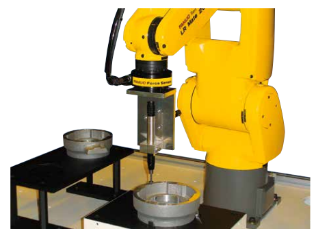
Force controlled deburring
